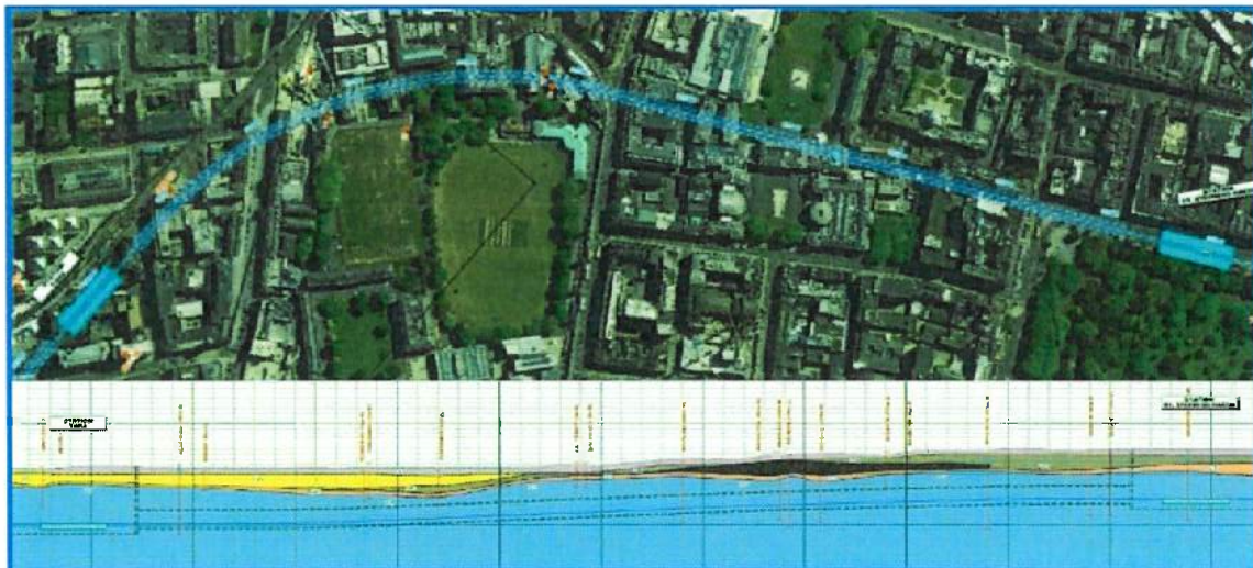
Figure 7. C8 Geological Section (ref. A5.13, Diagram 3.13; Geologic Profile for TBM Drive C8- Tara Station to St. Stephen's Green)
